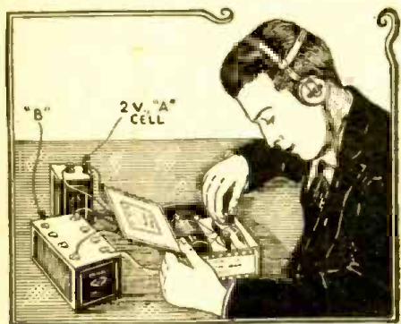
Fig. A. The complete receiver in the cigar box.
